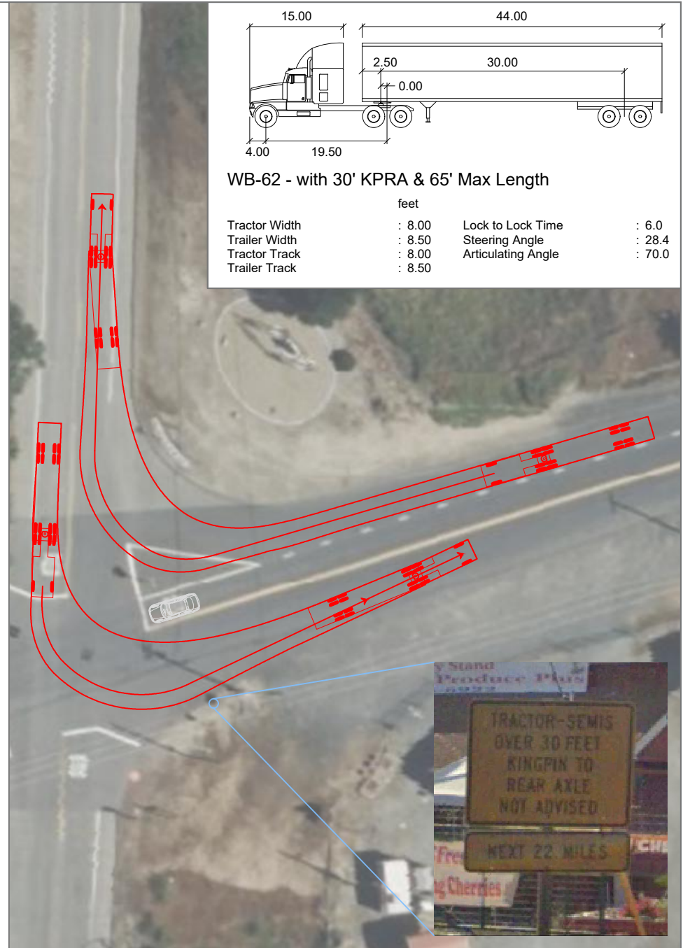
FIGURE 17 AutoTurn Analysis - WB 62 with 30-foot KPRA & 65' Max Length
