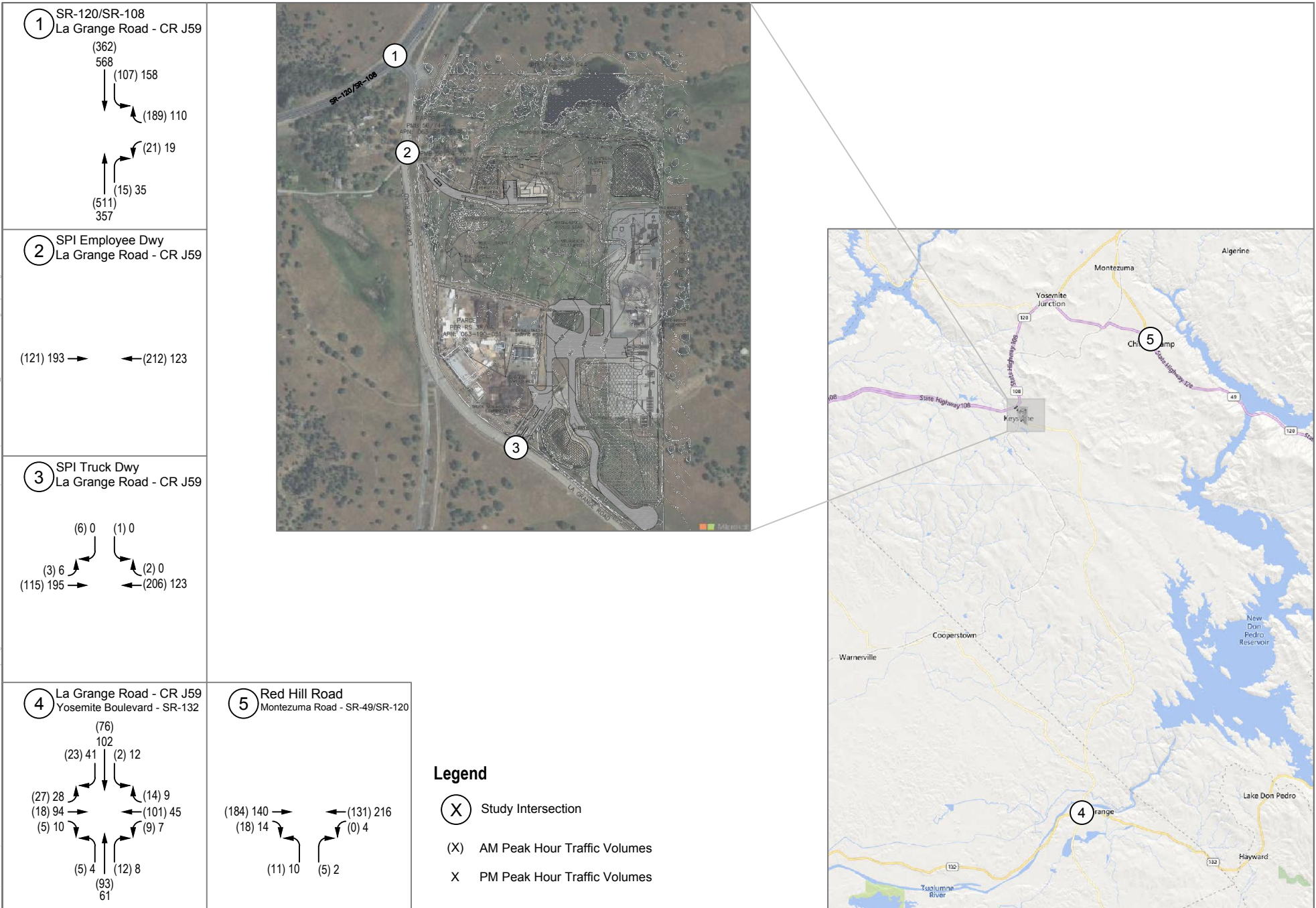
FIGURE 13 Opening Year (2025) Peak Hour Traffic Volumes Golden State Natural Resources Forest Resiliency Demonstration Project
